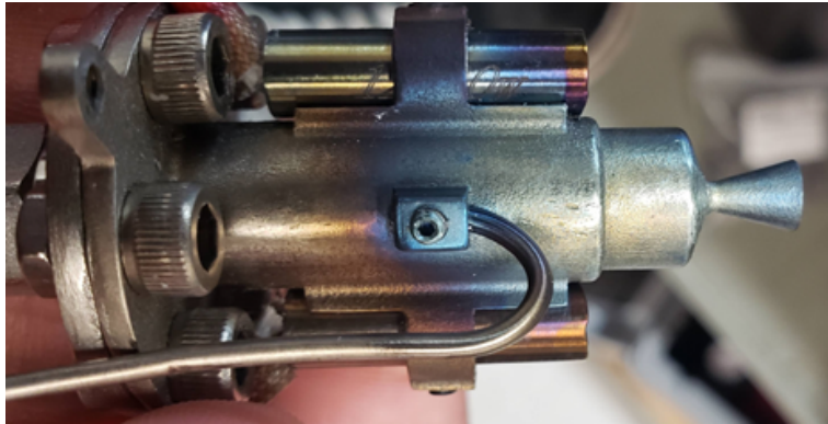
Figure 9. CTF-T with integrated nozzle and flanged compression-fitting inlet
