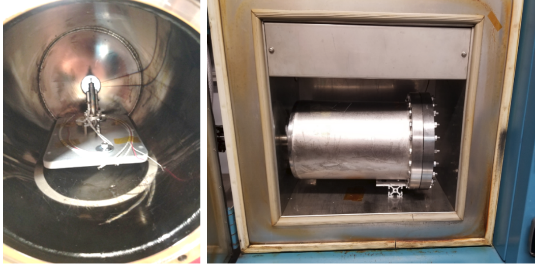
Figure 21. T-14 mounted to base plate ready and inserted into TVAC chamber.
