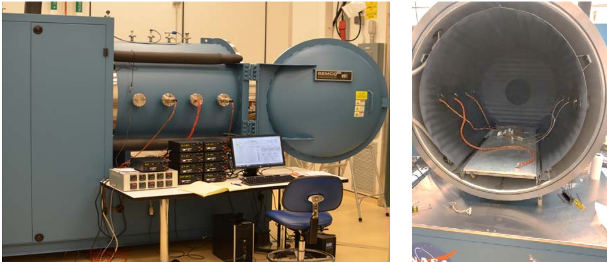
Figure 20. SPRL “blue” TVAC chamber. CAMFlow-3 mounted inside in right photograph.
