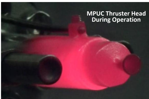
MPUC Thruster Head w/ Brassboard Propellant Feed System
