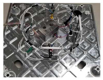
Mounting face of the GRASP Assembly Interface (ground demonstrator for PODS-scale module) is a monolithic base plate with GRASP mechanism (center), data connectors (centered around GRASP), and alignment groups (corners). Note the large amount of open volume available on the GRASP-IV monolithic base plate that is readily adjustable in size.
