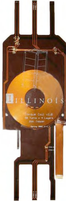
Figure 16: Torque coil implemented on flexible printed circuit.
