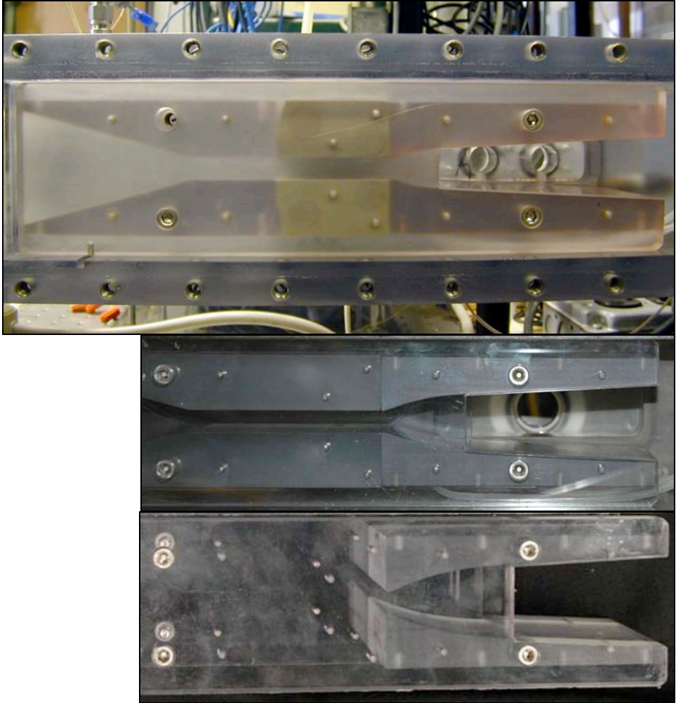
Figure 6. Photographs of the different nozzles tested to examine the effect of Mach number on the gain performance of the system: geometric Mach numbers of (a) 2.4, (b) 2.67, and (c) 3.0.
