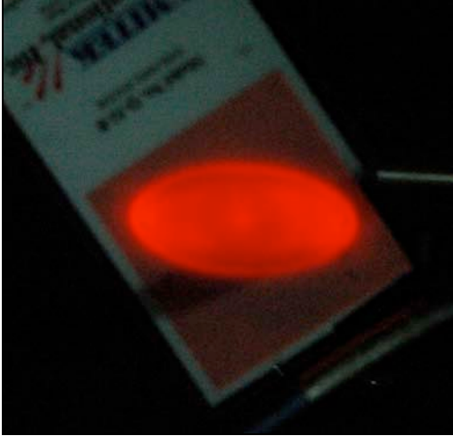
Figure 11. Photograph showing the 3.5 cm wide, elliptically-shaped 4.5 W laser beam on a thermal image card.
